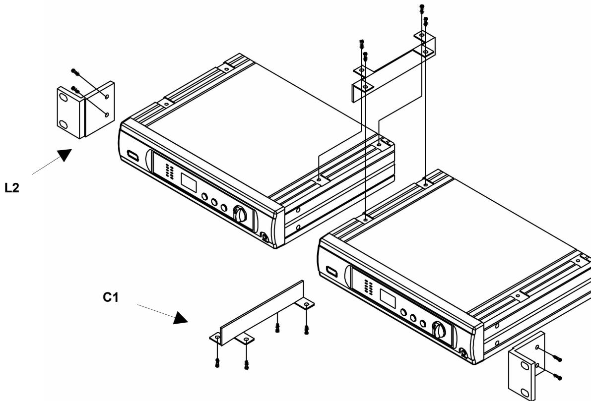
To mount a receiver in a 19" standard rack by using 2 L type long metal racks (L1).
