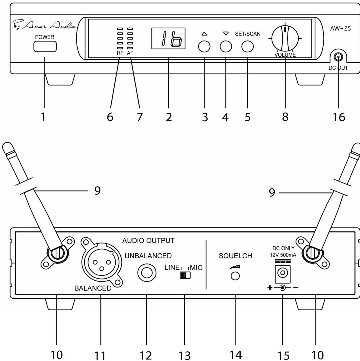
1. Power: Press for 2 seconds to power the receiver on or off.
