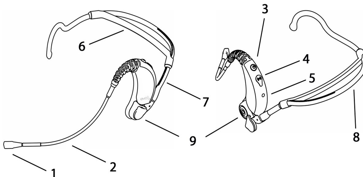
1. Microphone Element: Shown without the windscreen. Always be sure the side with the yellow dot is toward the mouth. In the event that you experience a low audio level with excessive feedback, check the direction of the microphone element. **DO NOT** twist the element.
